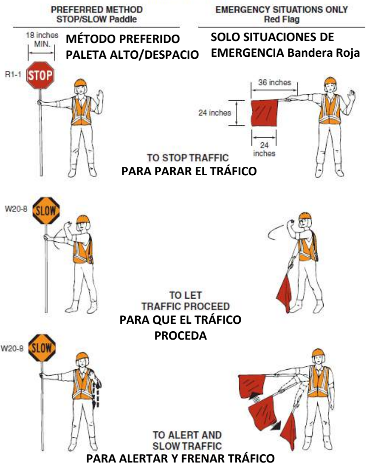
Figure 6E-3. Use of Hand-Signaling Devices by Flaggers
